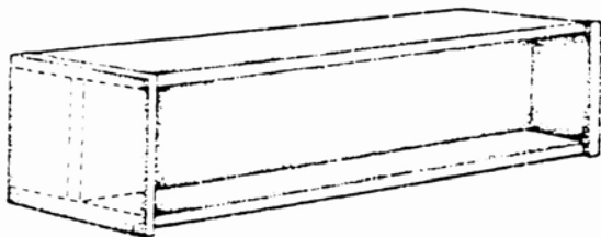
Figure G Beam with End Supports
